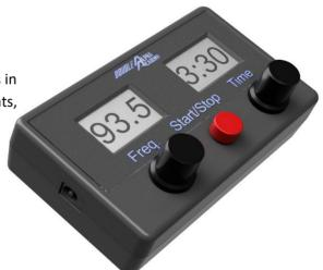
The Right knob on the controller sets the unit's shutdown delay from 30 seconds to 4 minutes. Most Small Primer tubes fill within 1.5-2.5 minutes, while Large Primer tubes may take a bit longer. Toggle between fine and rough run-time adjustments by pushing the knob in.
